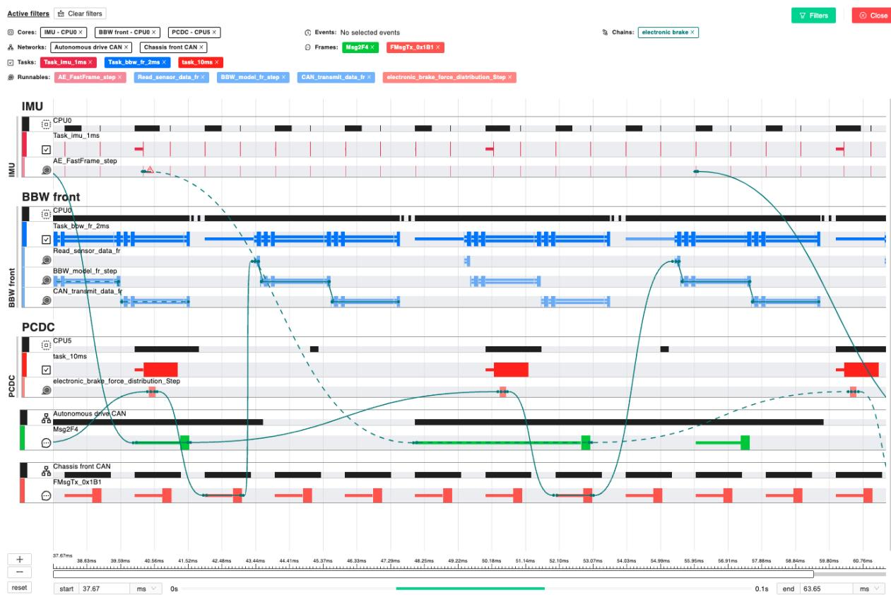
Failing event chains are shown with a dotted line, and, by clicking on the line, it is possible to get more details about it. The gantt chart shown by clicking on the action button near an event chain, abstracts all the information about the simulation to focus on the specific timing requirement. However, it is possible to get the whole simulation data by clicking the “Show Timing Gantt” button.
